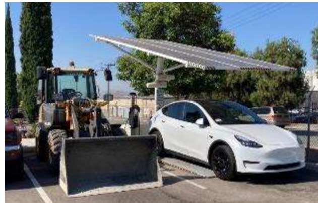
Figure 16: L25 Charging on Solar Charger
