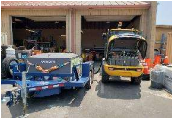
Figure 15: L25 Being Charged by Mobile Battery Bank
