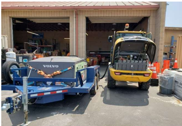
Figure 2 – L25 Being charged by Mobile Battery Bank
