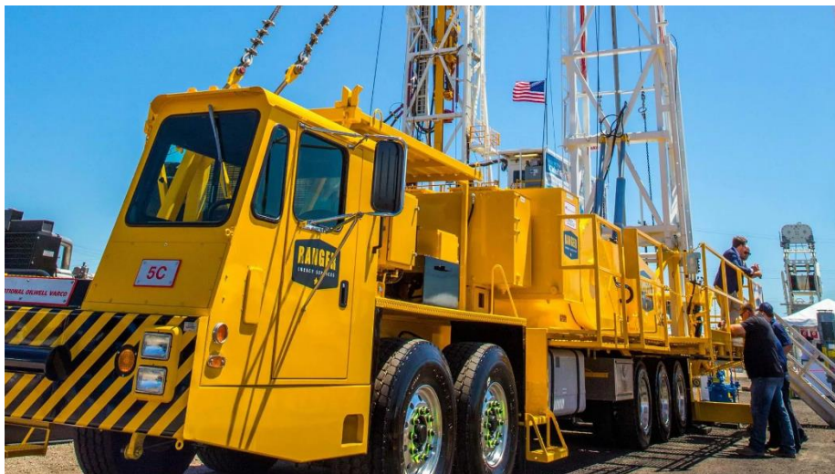
Figure 1: A Workover Rig Used in the Oil Production Field
