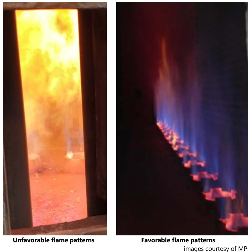
Figure 1-3 Unfavorable and favorable flame to flame interaction and coalescence.
