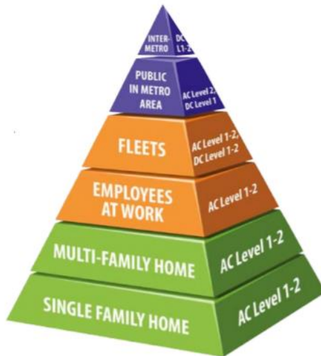
Figure 1. This pyramid illustrates how likely PEV drivers are to need and use each type of charging infrastructure. Image from Argonne National Laboratory.
