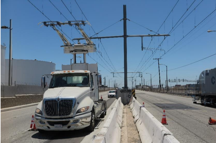
TransPower Catenary Truck on the OCS Track
