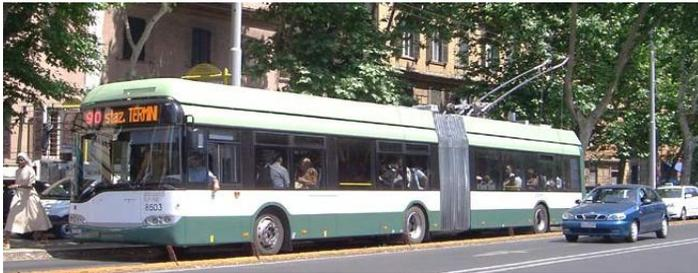
Figure 4 Dual-Mode Battery Electric Transit Bus (Rome)
