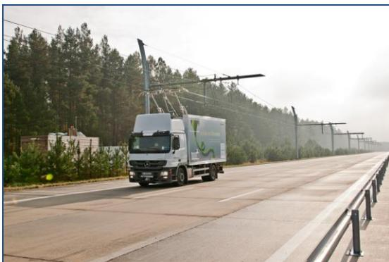
Figure 5 Truck Catenary (Siemens)
