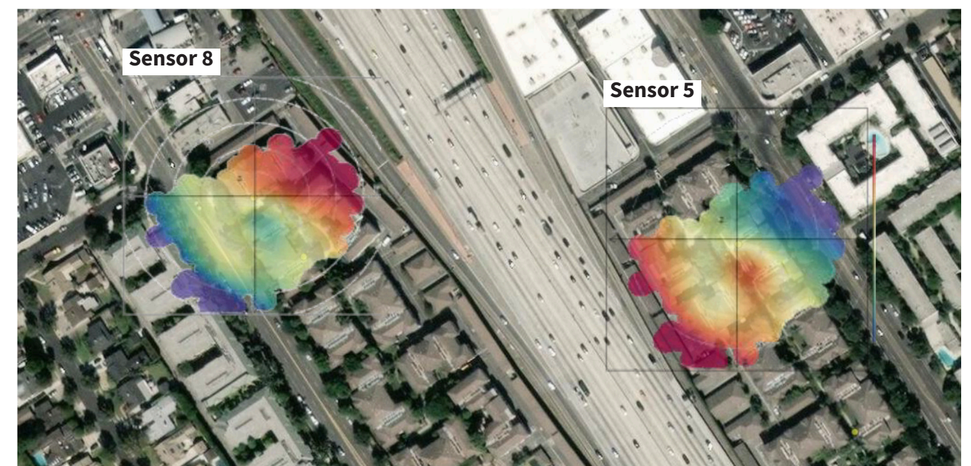
Fig. 6: polar plots of June 2018 weekday morning \text{PM}_{0.3} at Sensor 5 (Sepulveda side) and Sensor 8 (Sawtelle side). Plots were created by subtracting the Sensor 8 PM from Sensor 5 to control for ambient levels and comparing these readings to wind direction and speed recordings. Warmer colors indicate the direction of the emissions source. Here, we can see that \text{PM}_{0.3} is coming from the freeway, and is slightly higher on the Sawtelle side than the Sepulveda side.
