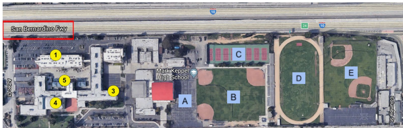
Figure 1. Aerial view of Mark Keppel High School acquired from Google Maps. Yellow dots indicate the location of the four PurpleAir sensors on campus. Sensors are named SCAP 1, 3, 4, 5 based on their ID number in the PurpleAir database. SCAP 1 is 179 ft. from the San Bernardino Freeway; SCAP 3 is 397 ft. from the San Bernardino Freeway; SCAP 4 is 490 ft. from the San Bernardino Freeway; SCAP 5 is 328 ft. from the San Bernardino Freeway. Blue squares indicate athletic facilities: basketball court (A), open field (B), tennis court (C), track (D), baseball field (E).
