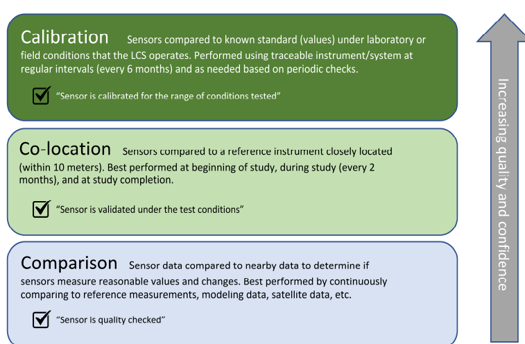
Figure 5. A schematic of typical levels of validation of sensors and instruments
