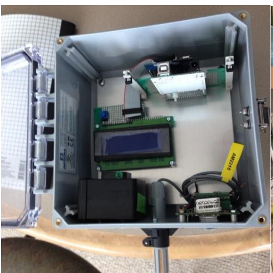
Figure A.1. Sensor pod assembly
