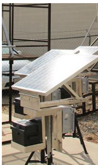
Figure A.2. Fully assembled pod with solar panel, battery cell, and tripod.
