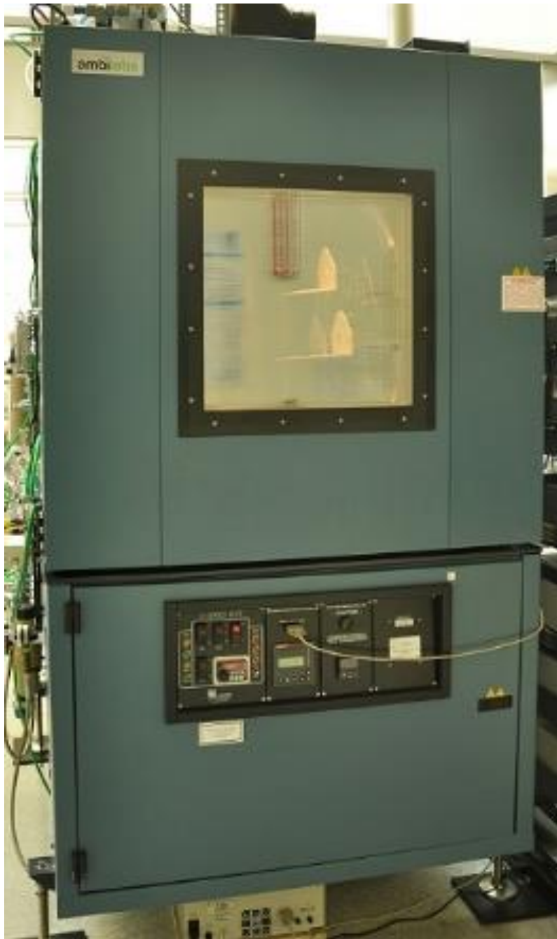
Figure 1. AQ-SPEC's laboratory environmental Chamber 1 used for VOC sensor testing
