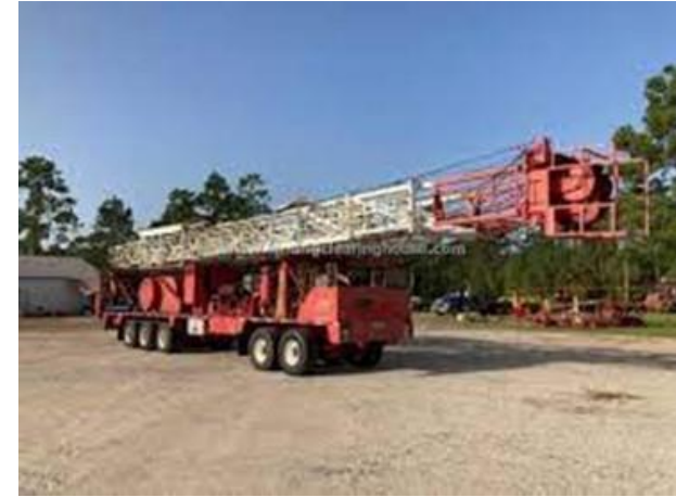
Example of a Workover Rig
