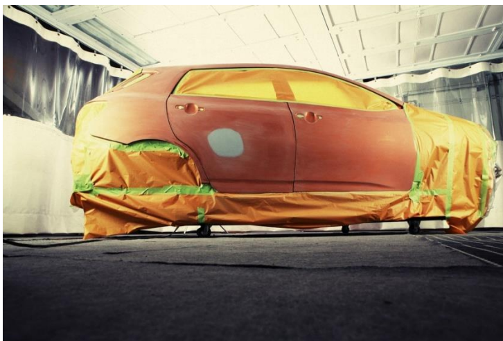
Figure 5f-1: Auto body repair shop painting a motor vehicle
