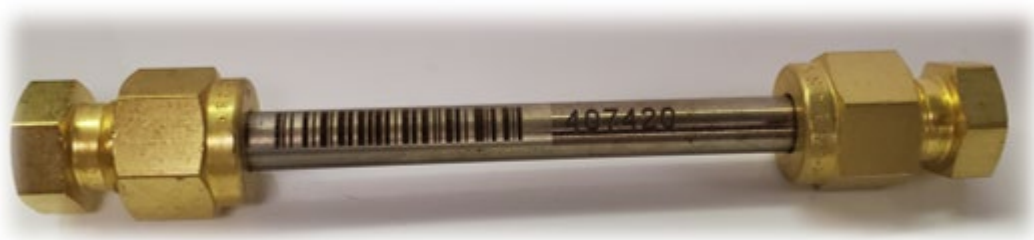
Figure 4 - Thermal Desorption Sample Tube with Brass Caps
