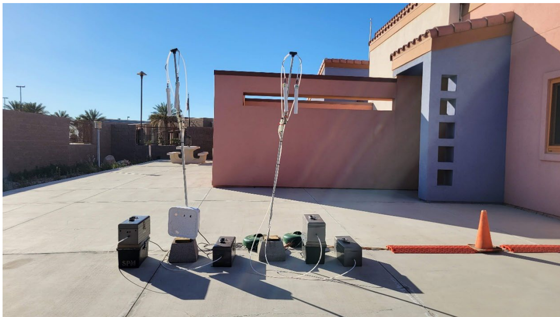
FIGURE 2 - SAMPLER AT THE MECCA FIRE STATION SITE
