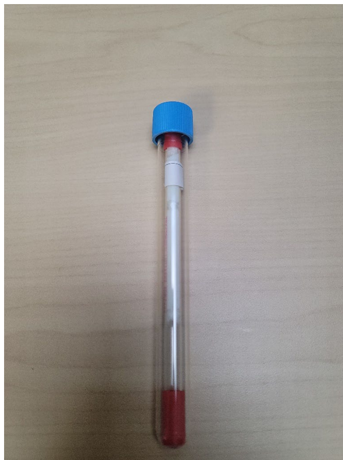
Figure 5 - XAD Cartridge in Culture Tube
