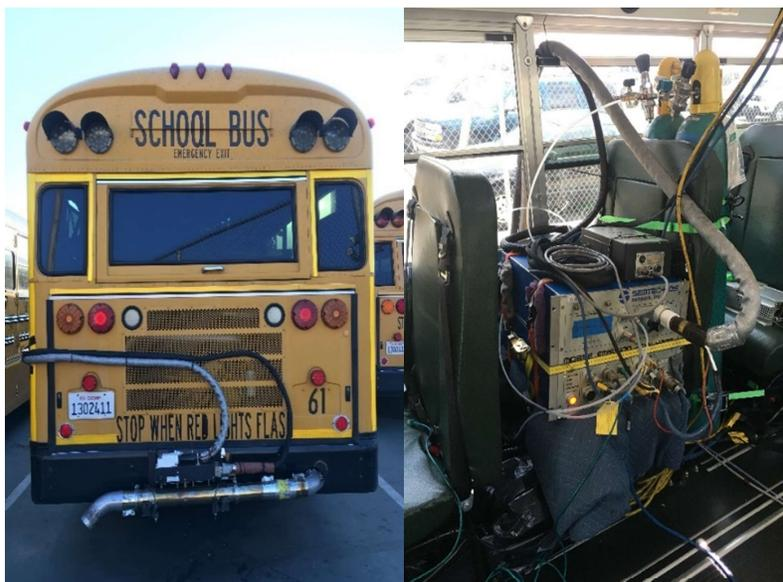
**Figure 4: PEMS Equipment Install on School Bus**
