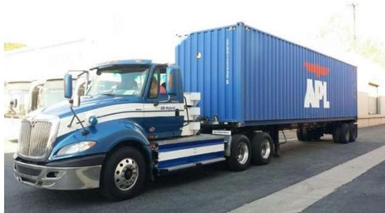
*Figure 2: eTruck™ 1 with 80,000 lbs GCWR Trailer*
