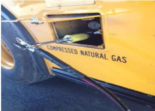
Figure 2: Type D CNG Bus Refueling
