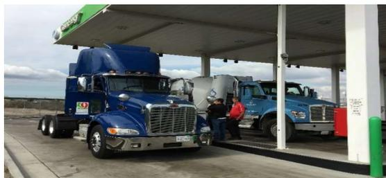
**Figure 3: Pac 9 Class 8 with ISX12N Refueling with CNG**
