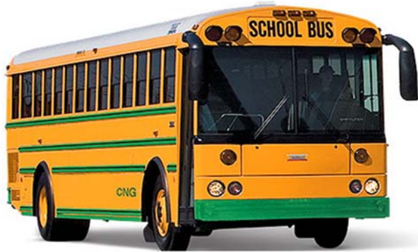
Figure 13: CNG Type D bus certified at 0.02 g/bhp-hr NOx
